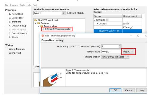
5. Click on the Wiring tab to see how the sensor is to be wired to the VOLT 100 series. Click OK after wiring the thermocouple.
